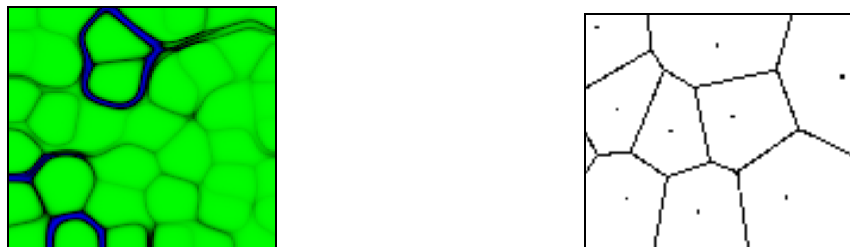
Figure 2. a - Example of self-organizing map. Each data point has a corresponding zone in the map and it is separated from the other points by a “valley” of variable width (e.g. near the top of the picture one cluster made of two patterns is clearly separated from the surrounding patterns by a wide boundary); b - Voronoi diagram. The separating lines do not have width unlike the self-organizing maps where the patterns are separated by boundaries of variable width
